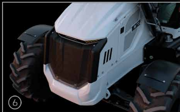
⑥ Durable engine front grille and protection bumper
